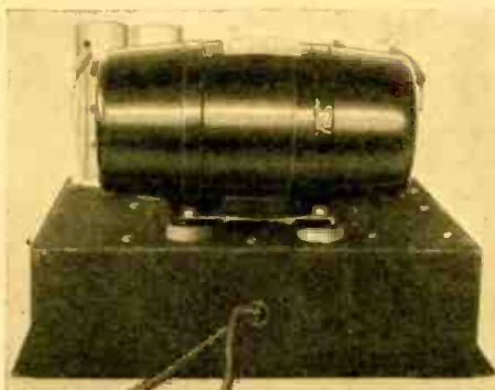
Back view of the Lafayette six-volt amplifier with the back housing removed to show the special six volt dynamotor and its soft rubber mounting.
