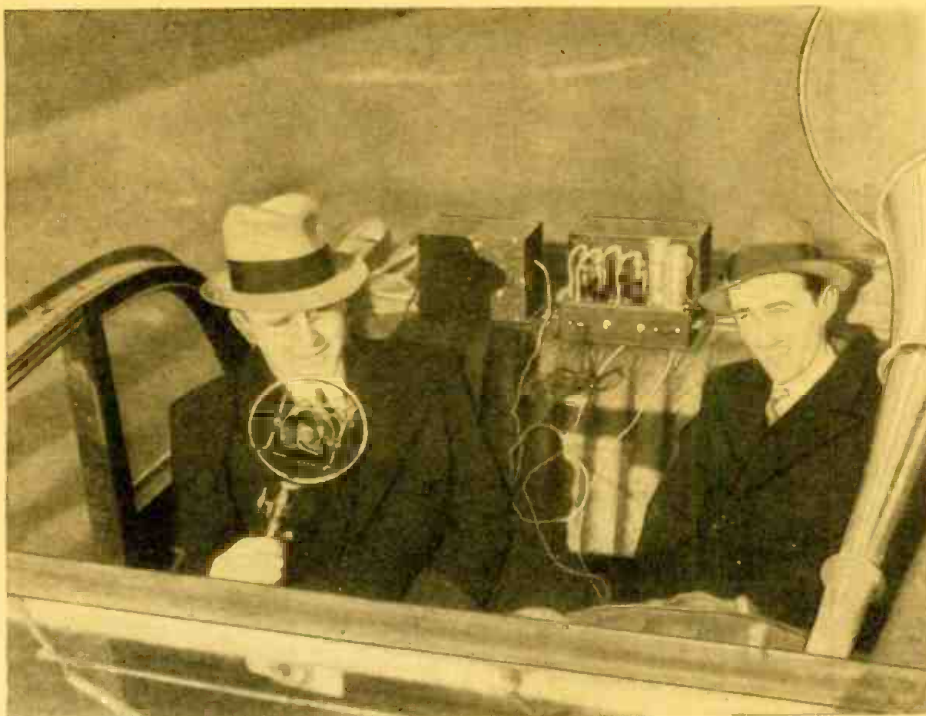
The authors operating the amplifier as part of a small public-address amplifier. Mr. Shortt is at the microphone, Mr. Lester is in the back. The mike control box and the amplifier itself are on the back seat. The loudspeaker is protruding from the right side.
