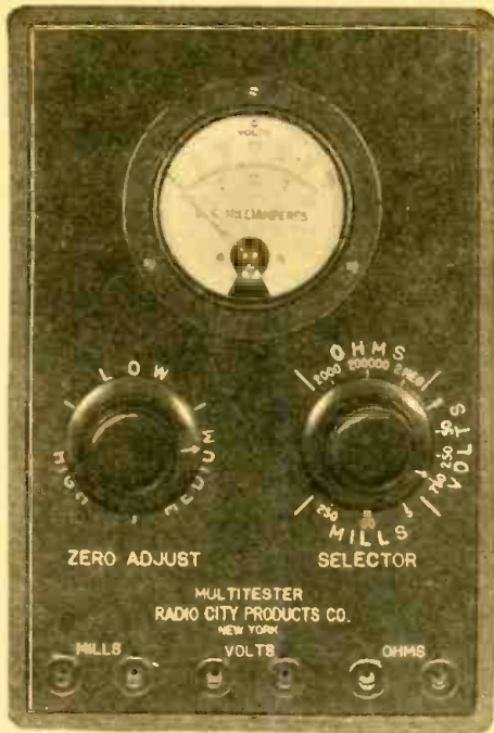
Panel view of the Multitester showing the location of all panel controls.
